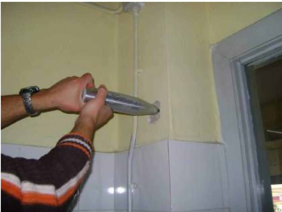
**Figura 66** – Sclerometria pilastro P/PT/11
