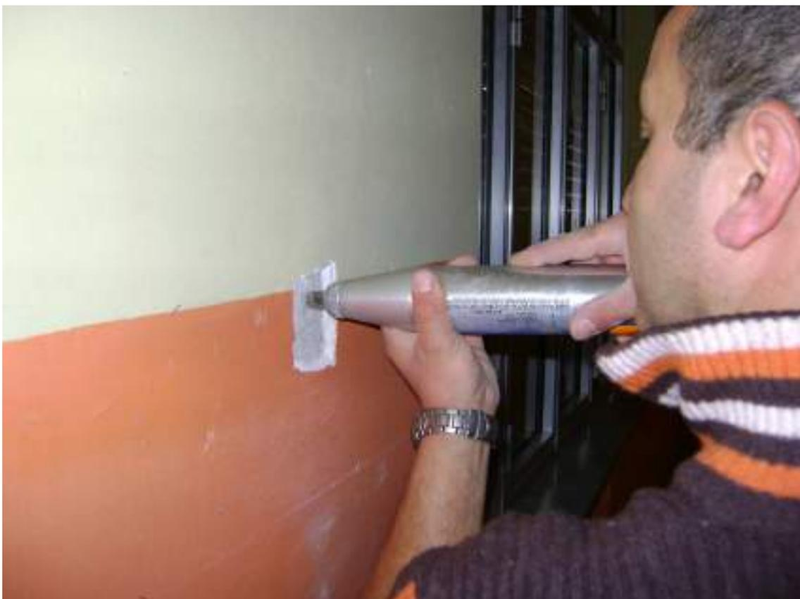
**Figura 60** - Sclerometria pilastro P/PT/16
