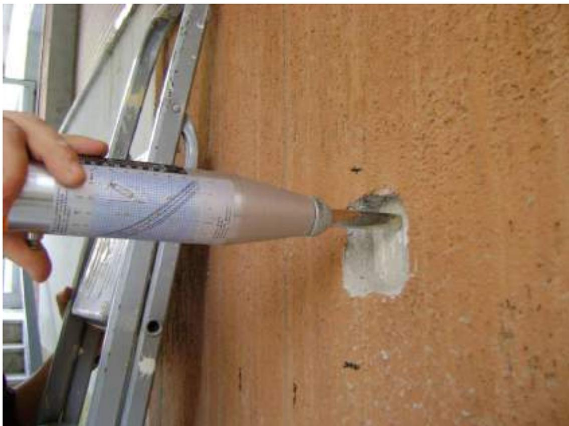
**Figura 62** – Sclerometria pilastro P/PT/17
