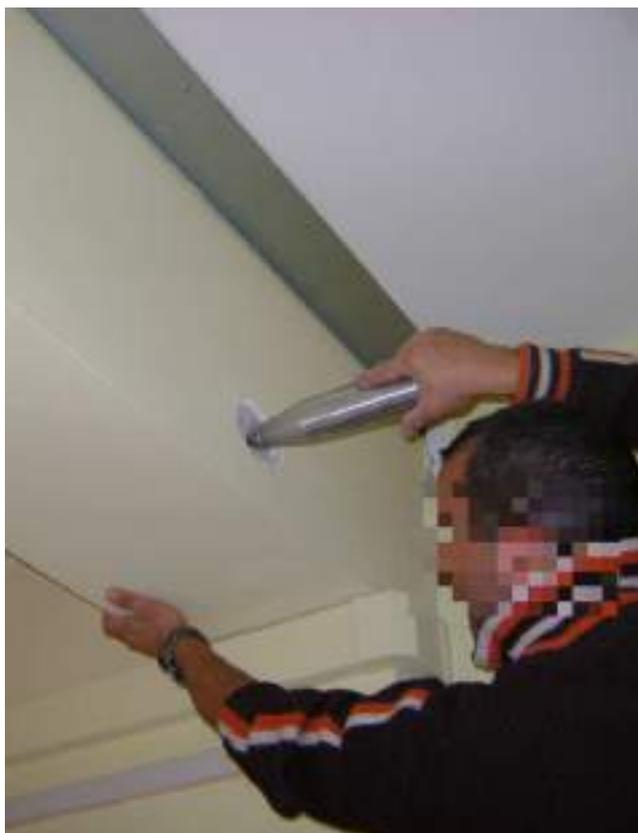
**Figura 11** – Prova sclerometria
