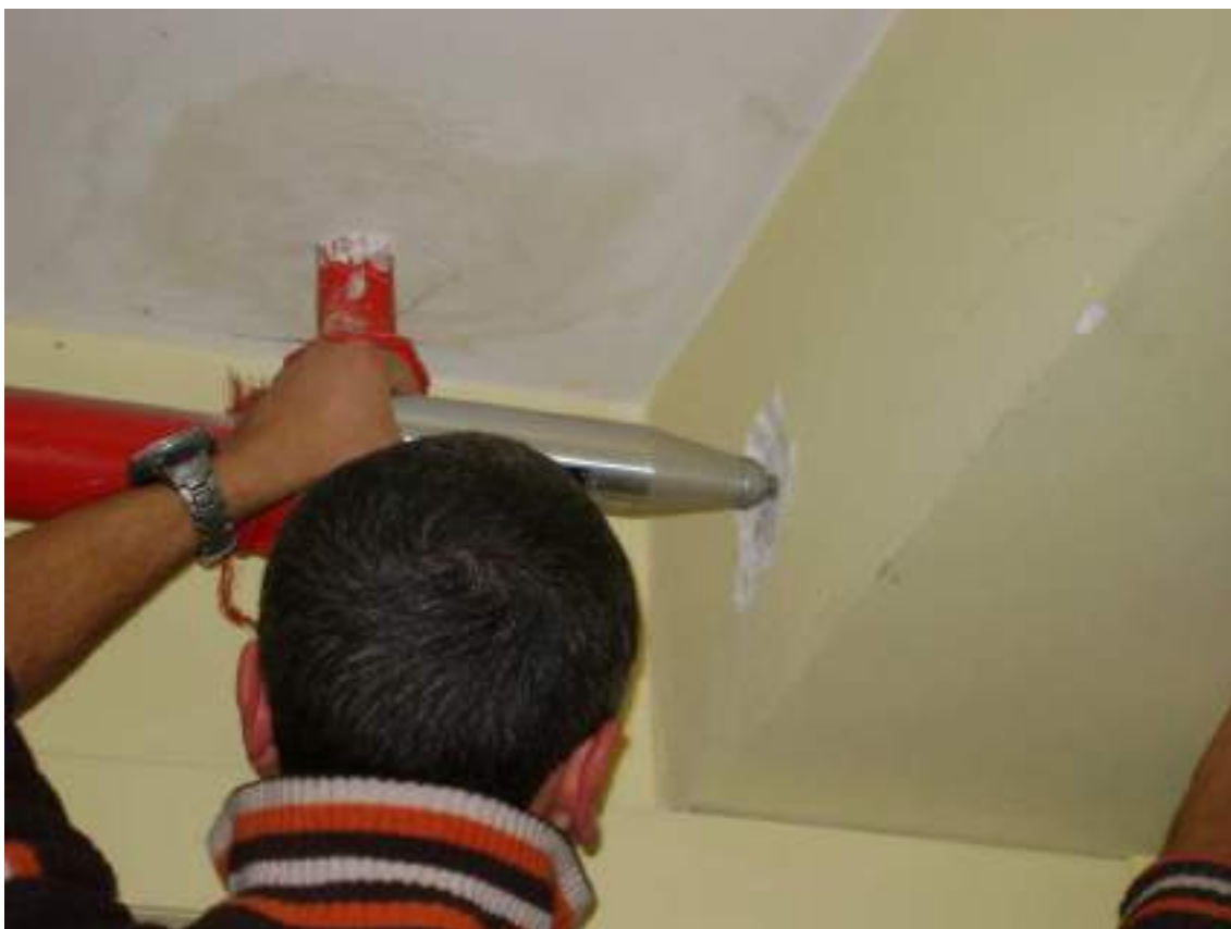
Figura 64 – Sclerometria trave T/PT/7-18
