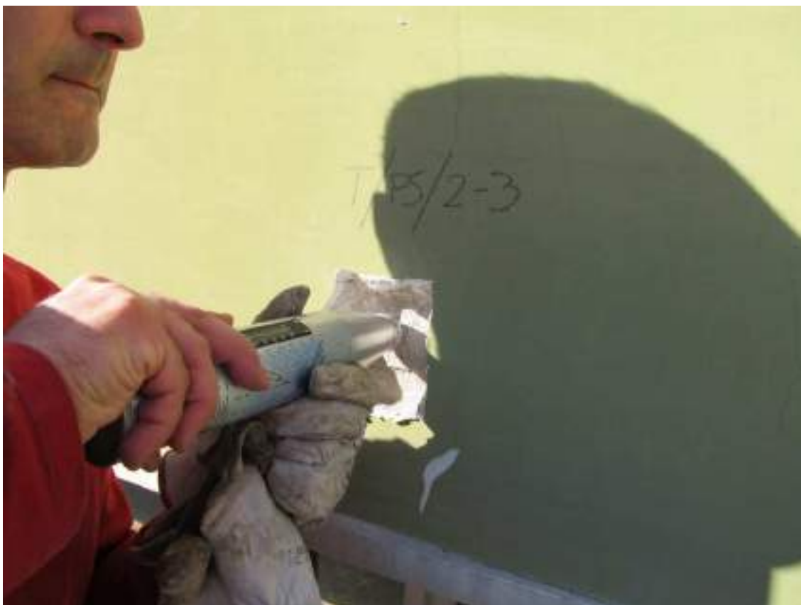
Figura 54 - Sclerometria trave T/PS/2-3
