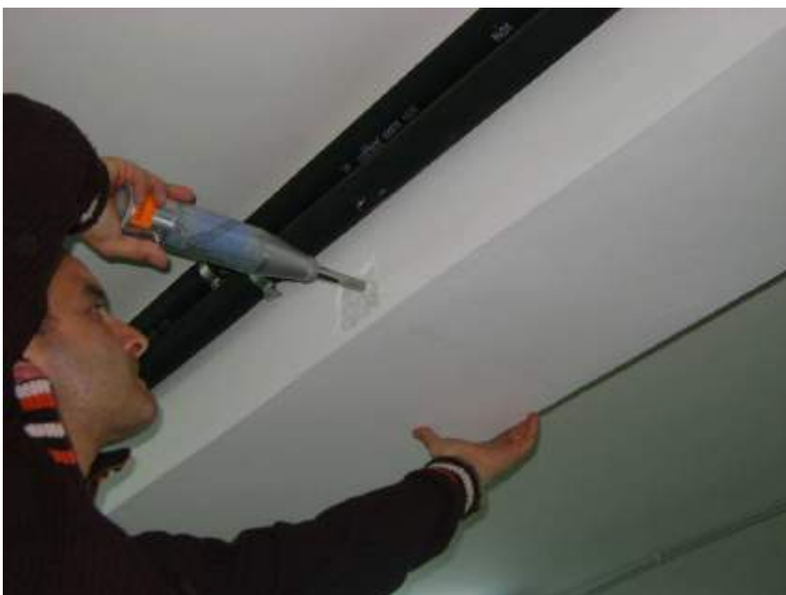
Figura 51 – Sclerometria trave T/PS/8-9
