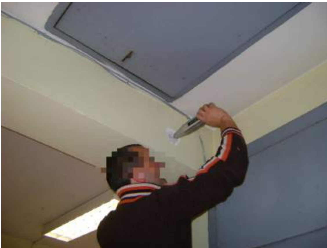
Figura 78 - Sclerometria trave T/1P/13-14
