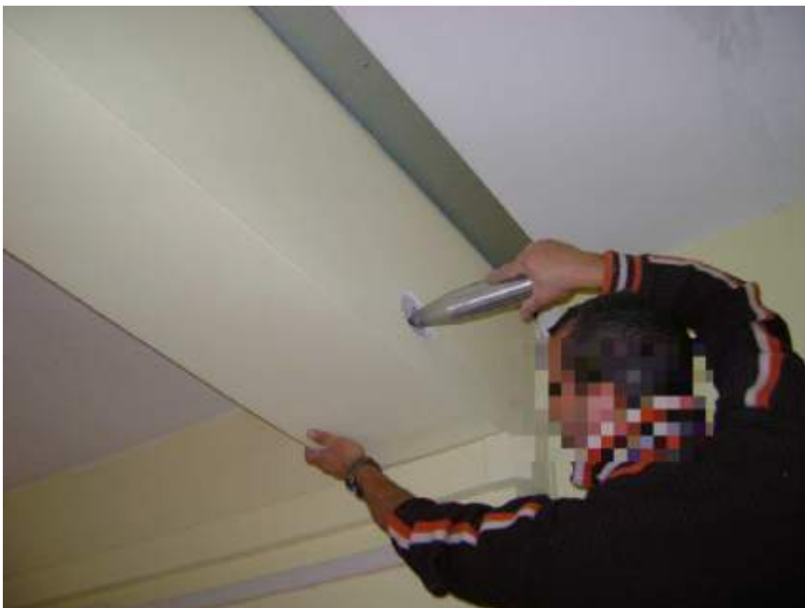
Figura 70 – Sclerometria trave T/1P/7-18
