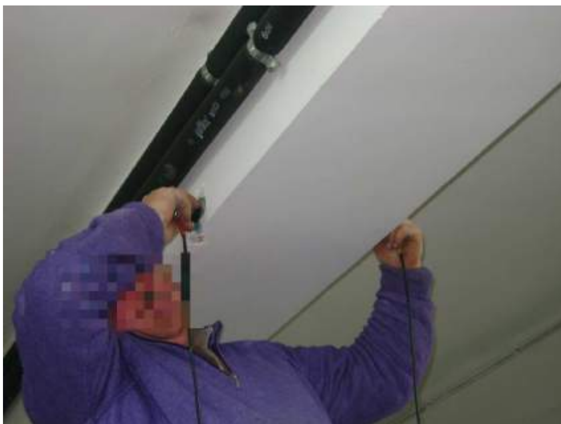
Figura 53 - Ultrasuoni trave T/PS/10-11
