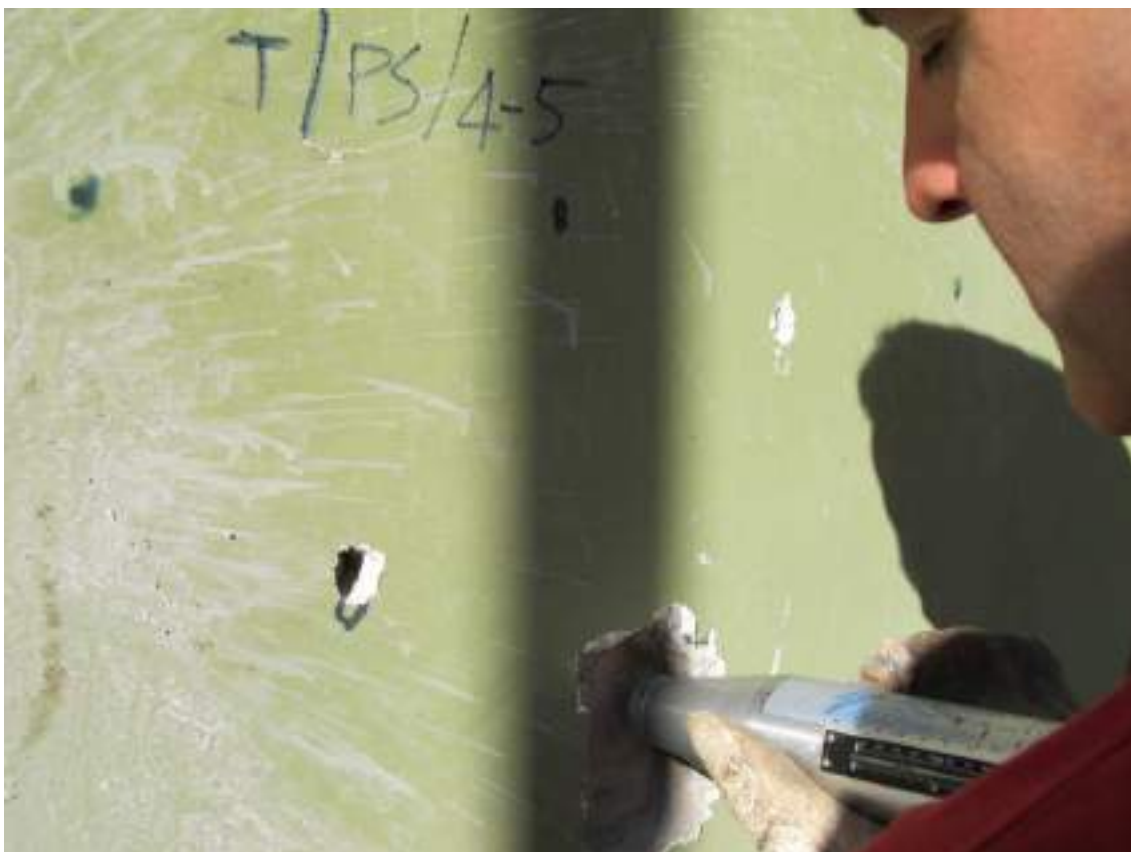
Figura 56 - Sclerometria trave T/PS/4-5
